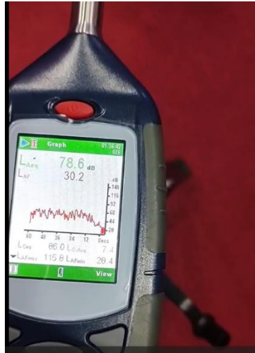
Fig. 7 Display of instantaneous sound level on the dB meter
