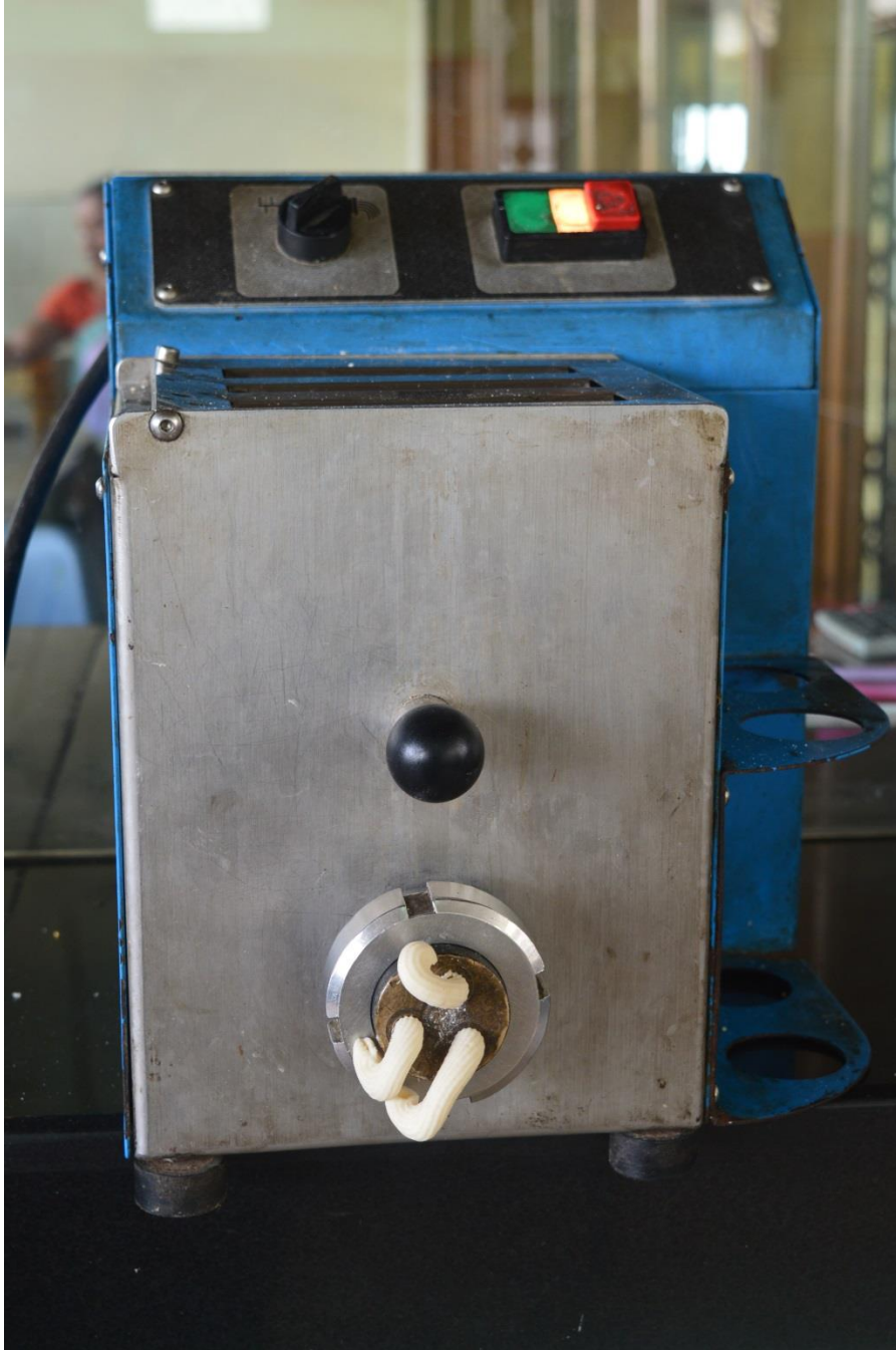
Fig. 17 Photograph of the extruder used for the preparation of pasta
